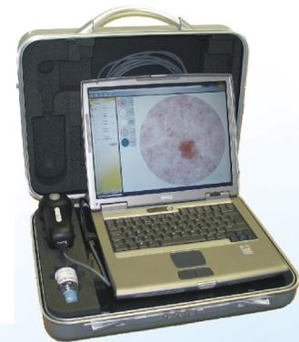
Figure 6 - A SIAscope packaged in a travel case
